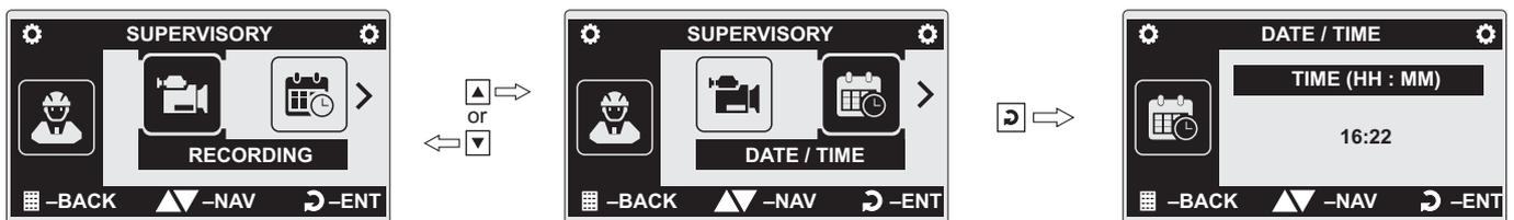
Once inside an access level, use the Up / Down keys to navigate and select a sub-level. Press Enter to access the parameters within the selected sub-level. The figure 3.4 above illustrates how to access the parameters within sub-level DATE / TIME under Supervisory access level.
