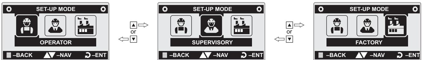
Use the Up/Down keys to navigate through the access levels. The currently selected access level is highlighted with an inverted colour scheme (white icon on a black background). Press Enter to confirm your selection.
