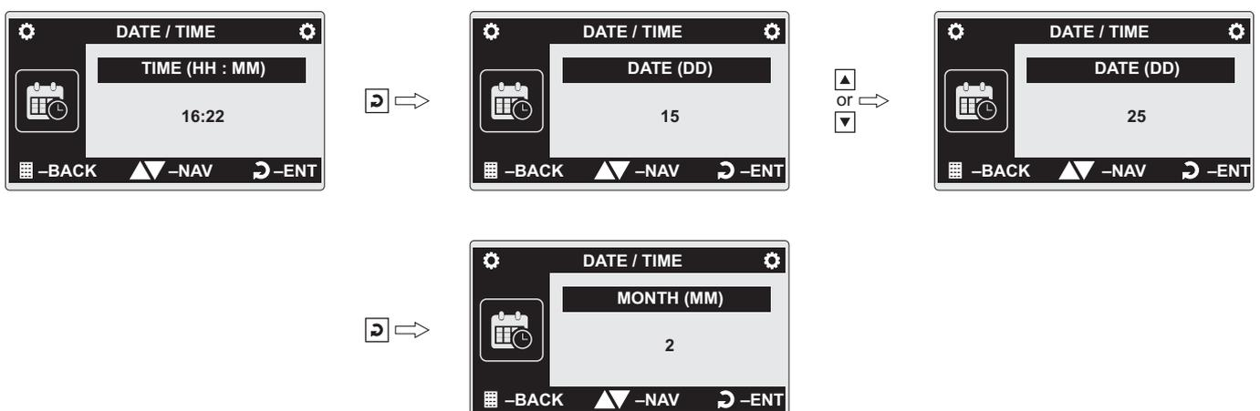
Once inside a sub-level, use Enter key to navigate through the parameters. Use the Up/Down keys to adjust the parameter value. Press Enter to save the modified value and proceed to the next parameter. The figure 3.5 above illustrates navigating to the parameters DATE (DD) within sub-level DATE / TIME under Supervisory access level and modifying its value from 15 to 25.
