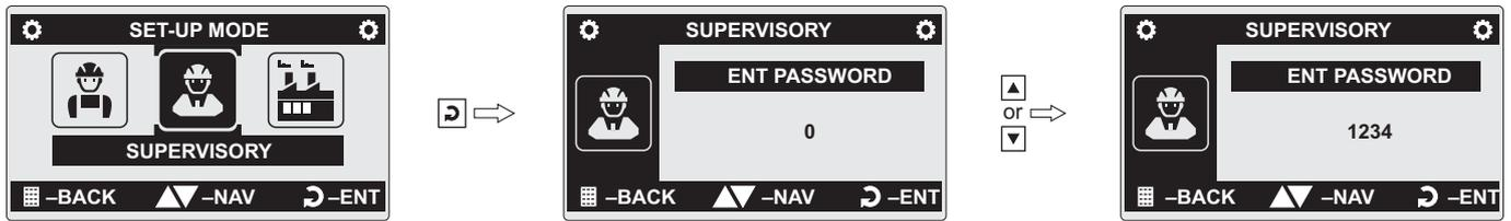
If the selected access level requires authentication, the **Enter Password** screen will appear. Use the **Up/Down** keys to enter the password (Figure 3.3). The default passwords are 1234 for Supervisory and 4321 for Factory access levels.
