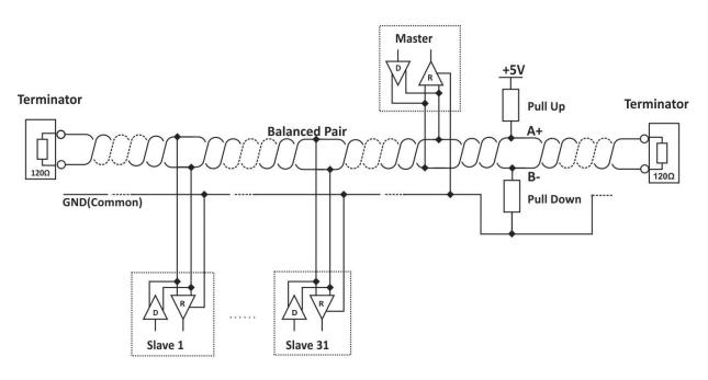
A daisy-chain (linear) topology and UTP/FTP cables for multiple sensors are strongly recommended. For proper operation of the interface, terminators (120 ohms resistors) must be installed at both ends of the bus. The device has a built-in 120 ohm resistor and to terminate the line, "Line-B-"and "Term" must be shortened.
