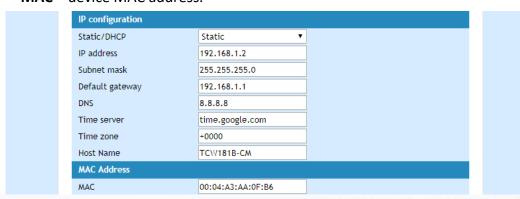
The good practice is to change the default IP address of the controller immediately after first power-on. This will avoid collisions if many devices are used on the same network. It may be necessary to clear the arp cache, each time you connect a new device to the network. This is done by typing arp -d in the command prompt of window computer.
