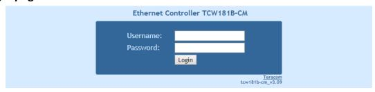
After opening the "Login" page, authorization data must be entered (by default username=admin, password=admin). It is recommended to change the username and password to prevent unauthorized access to the controller. Up to fifteen 1-byte UTF-8 symbols can be used.
