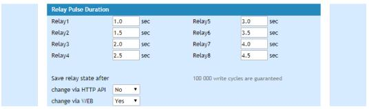
By default, relay state changes via the WEB interface are memorized in non-volatile memory. After the power on, the relay goes in its last state, before the power down.
