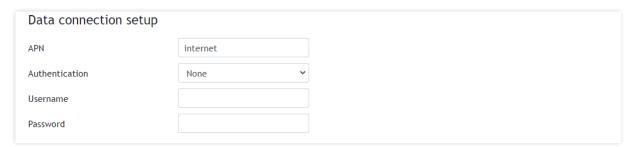
This setting can be different for each mobile operator. By default, APN (Access Point Name) is "internet". Some mobile operators may require also a username and password.
