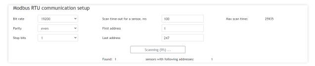
TCG140-4 supports MODBUS RTU over the RS-485 interface. All sensors connected to this interface should work with the same communication settings.
