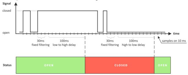
On the picture above low-to-high and high-to-low delays are set to 0.1 seconds.
