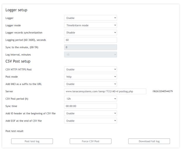
The logger works in three modes – Time, Alarm, and Time&Alarm. The mode specifies what initiates a record in the logger's memory.
