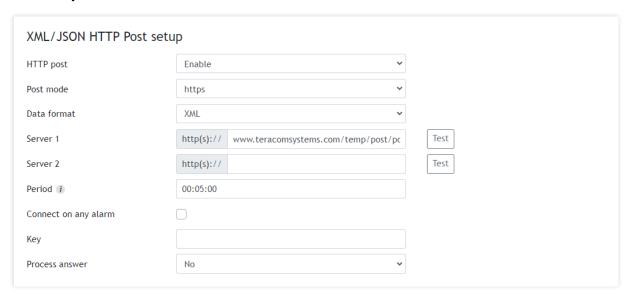
HTTP Post is used for periodically upload of an XML/JSON file to a server by HTTP/HTTPS requests (Post method). The file contains the current status of all monitored parameters and extra system information. The file format is chosen from the drop-down menu.
