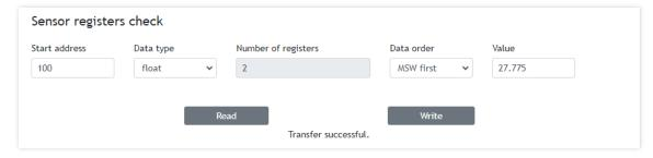
This part of the tool is used for general sensor register check.
