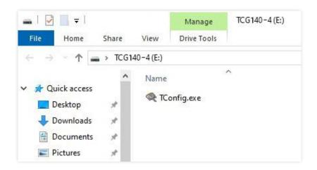
The only file stored on the mass storage is a tool called "TConfig". This tool enables communication between the TCG140-4 and PC. After starting the TConfig tool, the following program will appear:
