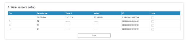
Detection of connected 1-Wire sensors is made either after power on or by the button "Scan". All found sensors are shown in ascending order refer to their unique ID number.
