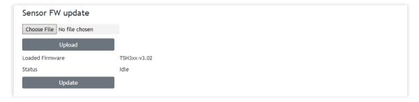
To arrange the FW update, the appropriate file should be uploaded to the sensor first and after this, the button "Update" should be pressed.
