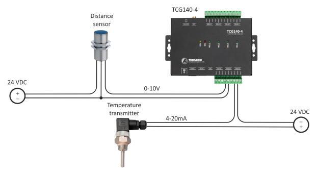
The maximum cable length for an analog input should be up to 30 meters.
