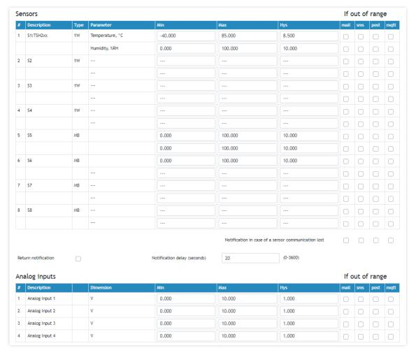
For every sensor two types of fields are presented – one for the trigger conditions ("Min", "Max", and "Hys.") and another one for the wanted action.
