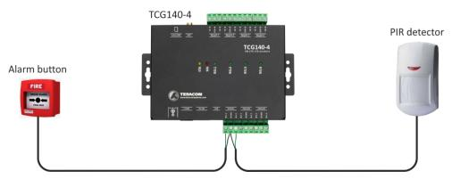
The maximum cable length for a digital input should be up to 30 meters.
