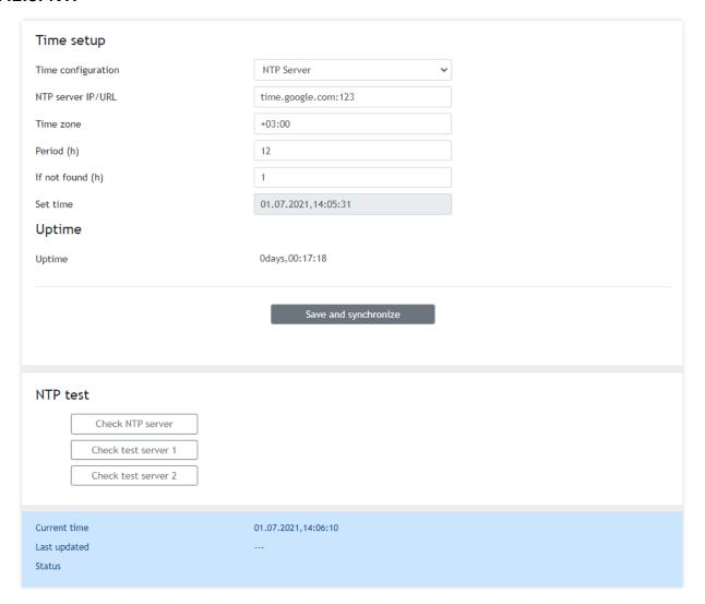
Internal RTC (real-time clock) of the module can be set either manually or automatically.
