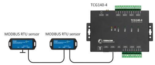
Interconnections are realized by UTP/FTP cables with RJ-45 connectors. The popular Ethernet wiring standard ANSI/TIA/EIA T568B is used.
