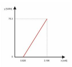
The sensor provides raw voltage values as output, but what we actually need is the corresponding relative humidity values. To achieve this, we use a multiplier and an offset. These two parameters allow us to calculate the relative humidity for any given voltage within the sensor's working range.
