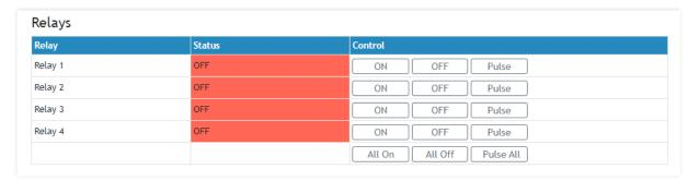
The section displays the current state of relays. Each relay can be activated either remotely or locally from the status of a monitored parameter. For locally activated relays a text describing the controlling parameter is displayed rather than buttons.
