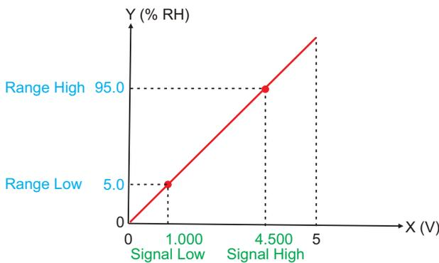
Presume the humidity is to be measured with 0.1 Resolution, that is 0.0 to 100.0 %.
