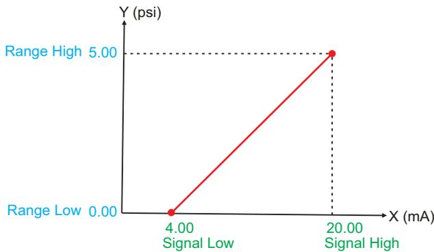
Presume the pressure is to be measured with 0.01 Resolution, that is 0.00 to 5.00 psi.
