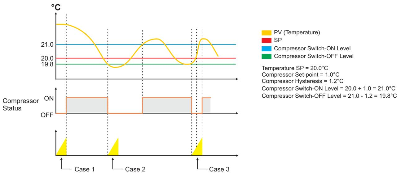
The figure above illustrates 3 cases. Case (1) illustrates power-up delay. In case (2); the time elapses before PV rises above the SP. The compressor is thus switched ON as soon as the PV rises above the SP. In case (3); the PV rises above the SP while the time delay is still in progress. The compressor is switched ON as soon as the delay time elapses.
