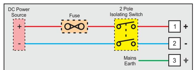
**For safety and enhanced electrical noise immunity, it is highly recommended to connect Mains (Utility) Power Supply 'Earth' to terminal 3.**
