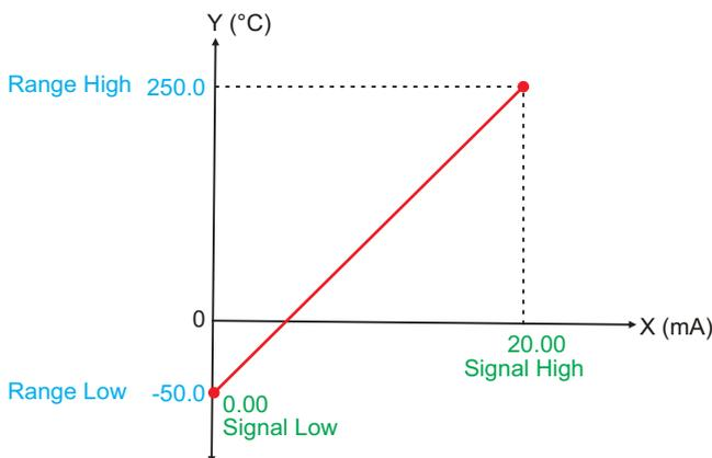
Presume the Temperature is to be measured with 0.1 Resolution, that is -50.0 to 250.0°C.
