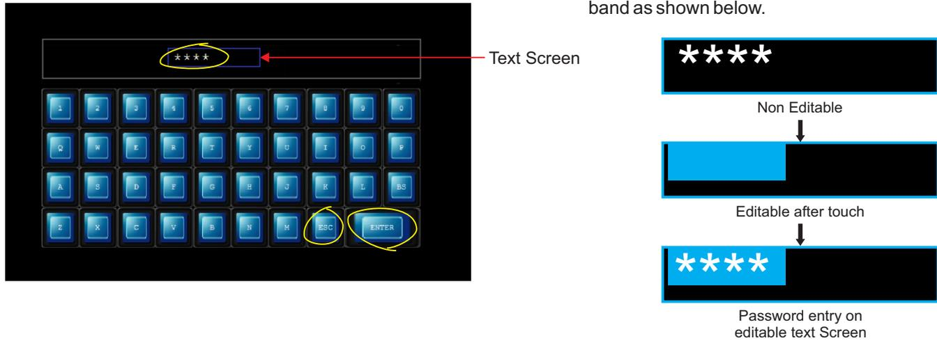
While the screen is editable, type 4 character password & then press ENTER Key. If the password is correct, the parameter setting screen opens up. Use ESC key (in case password is not known) to pop down the key pad.
