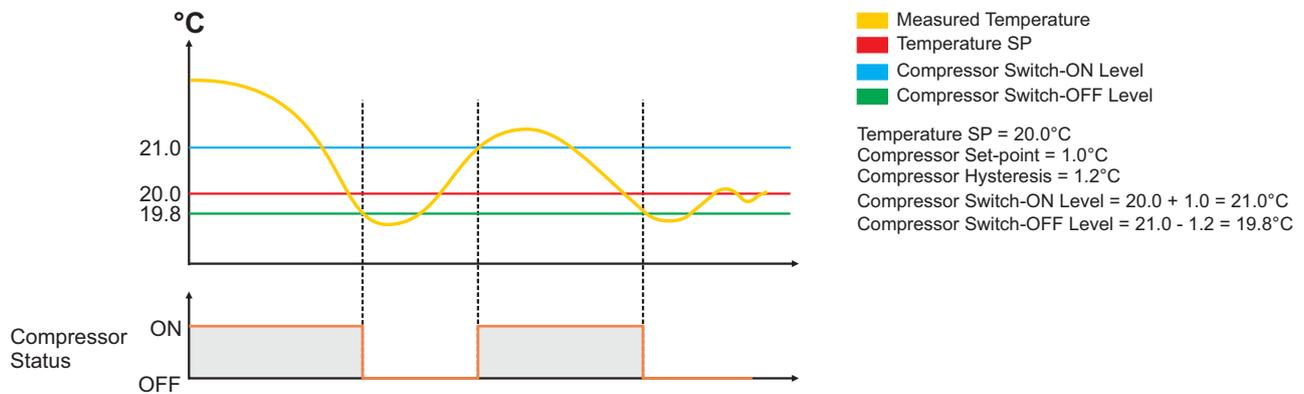
The compressor is turned ON if the equipment air temperature value is above the Temperature SP by an amount set by the parameter 'Compressor Set-point'. That is;
