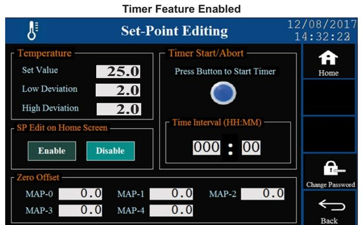
All the parameter settings, except Zero Offset, on this screen are Common for MAP-1 to MAP-4 Inputs.
