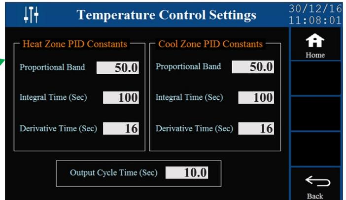
The control setting parameter screens depend upon the Control Action selected (On-Off Or PID).
