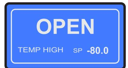
The Process / Event Alarm Status space on the screen may show one or more of the several messages listed in Table 2.2 depending upon the existence of active alarms. In case of co-existence of multiple active alarms, the messages are scrolled one after the other with an approximate time interval of 3 seconds. Also if there is no active alarm, the message space is blank.
