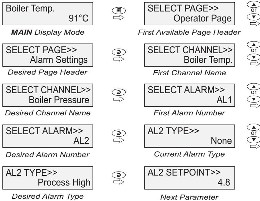
To exit the Set-up Mode and return to the MAIN Display Mode, press and release PAGE key.
