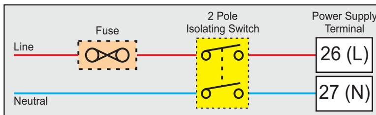
As standard, the controller is supplied with power connections suited for 85 to 264 VAC line supply. Use well-insulated copper conductor wire of the size not smaller than 0.5mm<sup>2</sup> for power supply connections. Connect Line (Phase) supply line to terminal 26 and the Neutral (Return) supply line to terminal 27 as shown in Figure 14.10. The controller is not provided with fuse and power switch. If necessary, mount them separately. Use a time lag fuse rated 1A @ 240 VAC.
