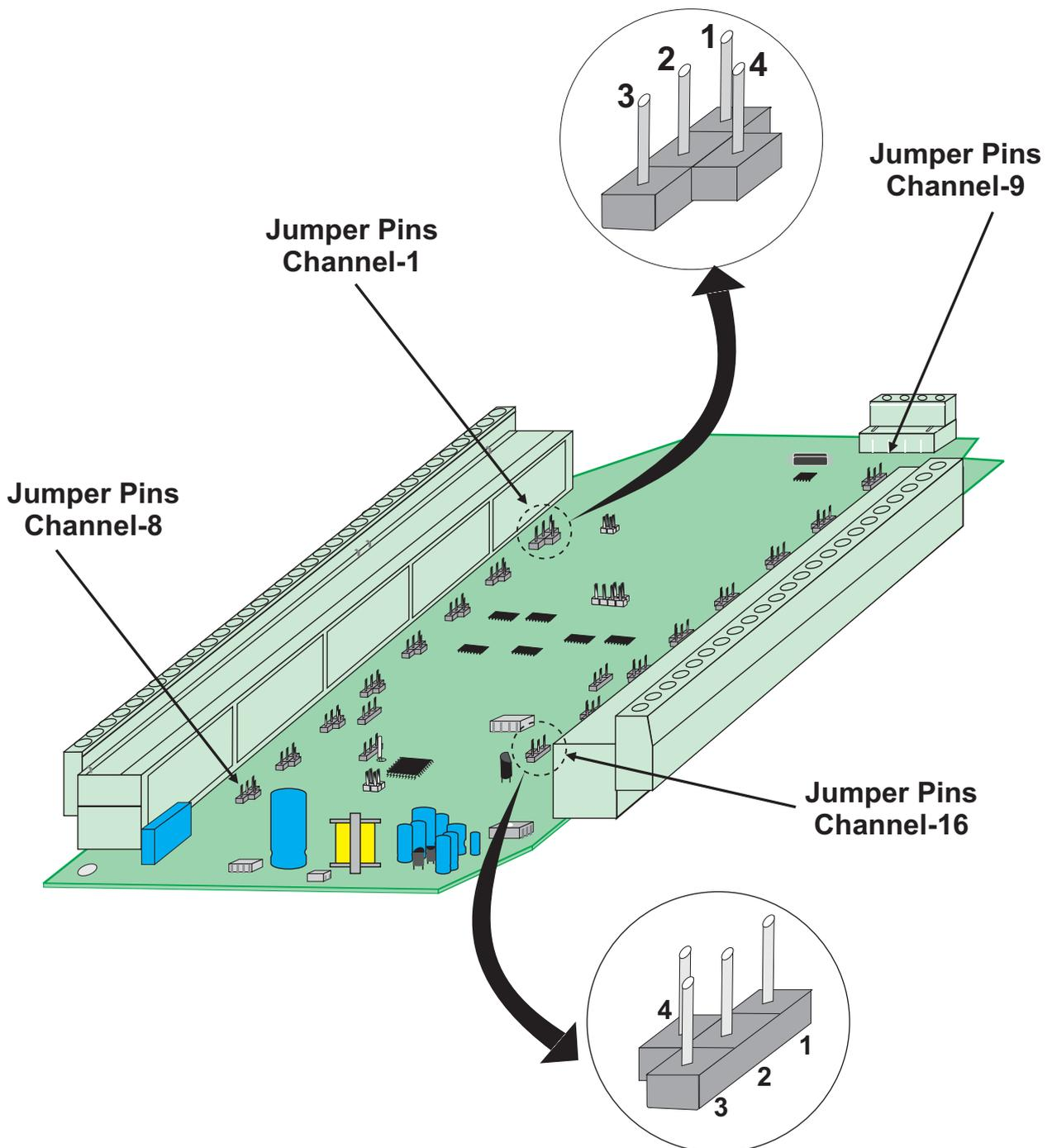
The jumper setting arrangement comprises of **Pins & Shorting-Link** as shown in the figure below. The figure also depicts how to mount the Shorting-Link for a particular jumper setting.
