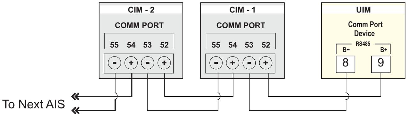
The UIM is connected to 1 or more CIM using RS485 Serial Communication Port. The wiring connections for interfacing the UIM with CIM is shown in the figure 16.1.
