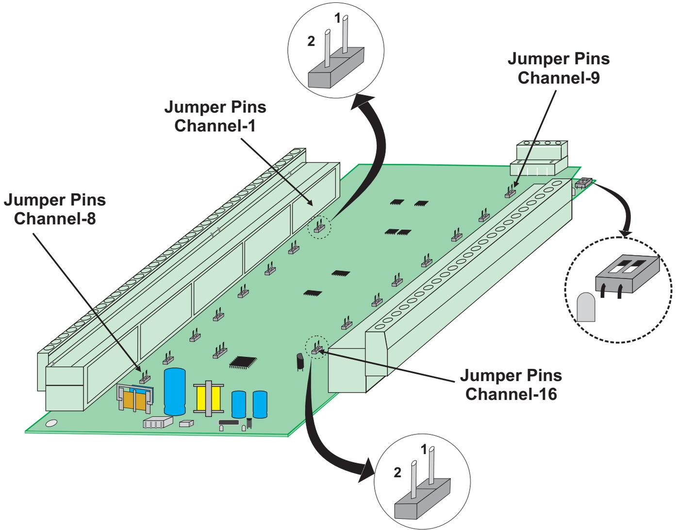
The jumper setting arrangement comprises of **Pins & Shorting-Link** as shown in the figure below. The figure also depicts how to mount the Shorting-Link for a particular jumper setting.
