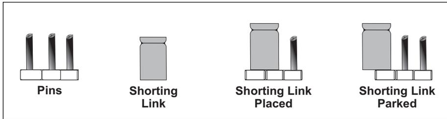
The figures below show the jumper settings for different input types.
