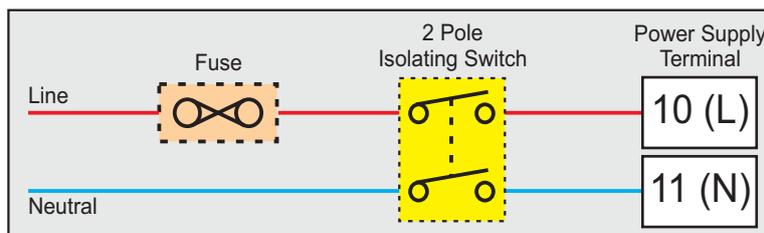
As standard, the recorder is supplied with power connections suited for 85 to 264 VAC line supply. Use well-insulated copper conductor wire of the size not smaller than 0.5mm<sup>2</sup> for power supply connections. Connect Line (Phase) supply line to terminal 10 and the Neutral (Return) supply line to terminal 11 as shown in Figure 14.7. The recorder is not provided with fuse and power switch. If necessary, mount them separately. Use a time lag fuse rated 1A @ 240 VAC.
