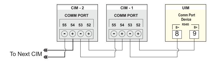
The UIM is connected to 1 or more CIMs using RS485 Serial Communication Port. The wiring connections for interfacing the UIM with CIM(s) is shown in the figure 17.1.
