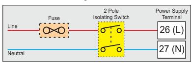
As standard, the controller is supplied with power connections suited for 85 to 264 VAC line supply. Use well-insulated copper conductor wire of the size not smaller than 0.5mm² for power supply connections. Connect Line (Phase) supply line to terminal 26 and the Neutral (Return) supply line to terminal 27 as shown in Figure 15.10. The controller is not provided with fuse and power switch. If necessary, mount them separately. Use a time lag fuse rated 1A @ 240 VAC.
