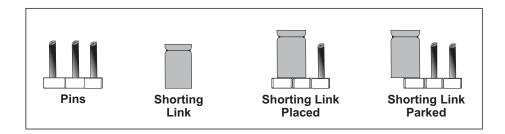
The figures below show the jumper settings for different input types.
