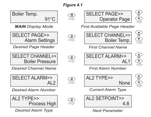
To exit the Set-up Mode and return to the MAIN Dispaly Mode, press and release PAGE key.
