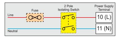
As standard, the controller is supplied with power connections suited for 85 to 264 VAC line supply. Use well-insulated copper conductor wire of the size not smaller than 0.5mm² for power supply connections. Connect Line (Phase) supply line to terminal 10 and the Neutral (Return) supply line to terminal 11 as shown in Figure 15.7. The controller is not provided with fuse and power switch. If necessary, mount them separately. Use a time lag fuse rated 1A @ 240 VAC.
