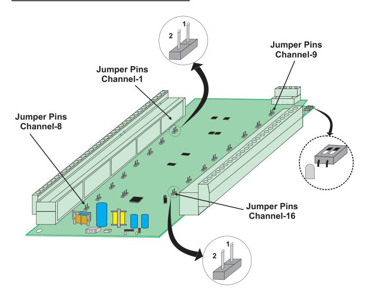
The jumper setting arrangement comprises of **Pins & Shorting-Link** as shown in the figure below. The figure also depicts how to mount the Shorting-Link for a particular jumper setting.
