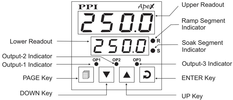
The front panel contains digital readouts, LED indicators and keys.
