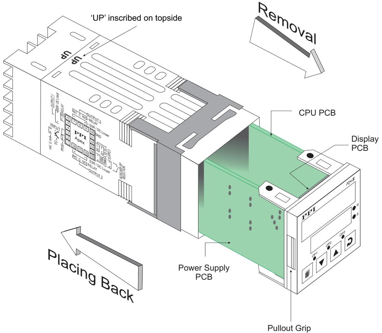
**Removing Assembly from Enclosure**
