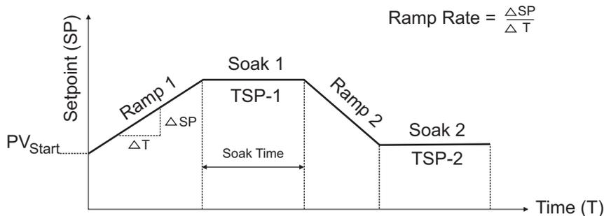
The controller provides a fixed-format, 8-segment Profile: 4 Ramp + 4 Soak; each Ramp followed by a Soak. The control algorithm continuously attempts to make PV equals SP and thereby the PV too follows the setpoint profile.
