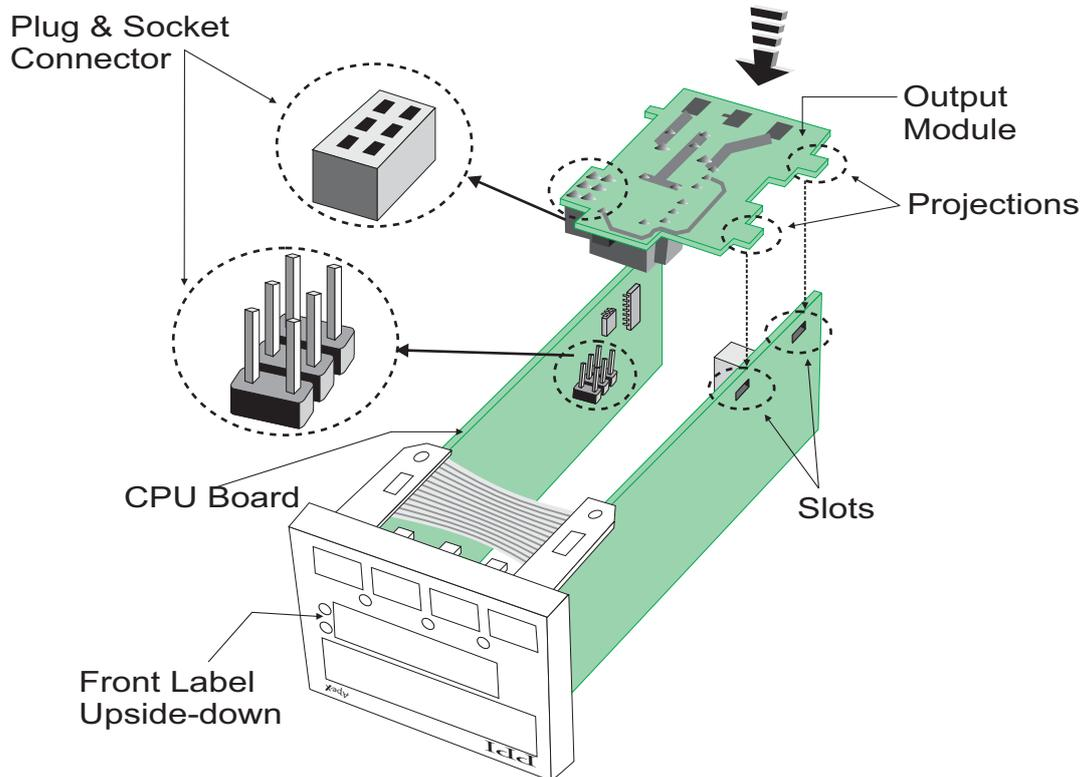
The plug for the Serial Communication or Auxiliary SP Selection module is located on the Power-supply PCB. The Figure 10.7 below illustrates how to plug-in the Serial Communication/Auxiliary SP module. To plug (or unplug) the module simply insert (or remove) the socket into (or from) the plug.
