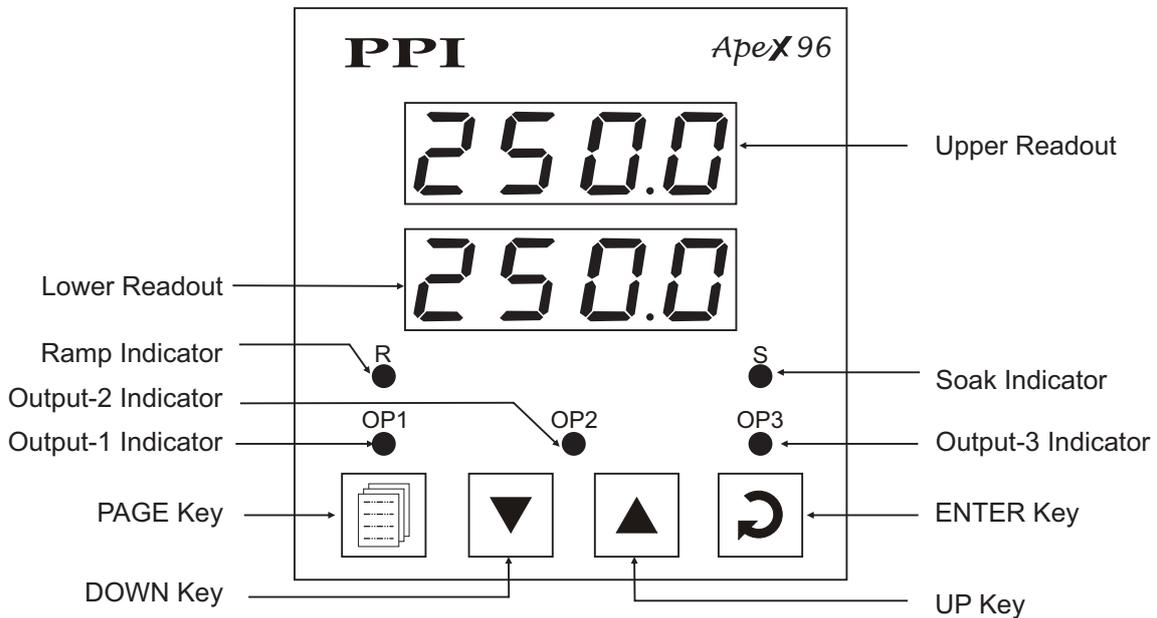
The front panel contains digital readouts, LED indicators and keys.
