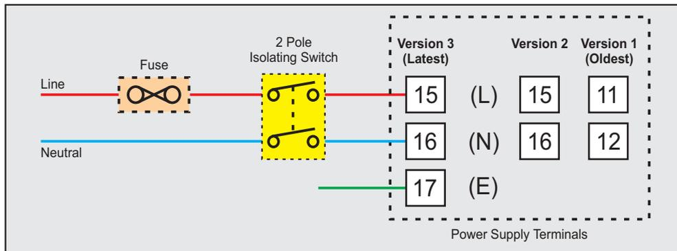
As standard, the indicator is supplied with power connections suited for 85 to 264 VAC. Use well-insulated copper conductor wire of the size not smaller than 0.5mm<sup>2</sup> for power supply connections ensuring proper polarity as shown in Figure 10.6. The indicator is not provided with fuse and power switch. If necessary, mount them separately. Use a time lag fuse rated 1A @ 240 VAC.
