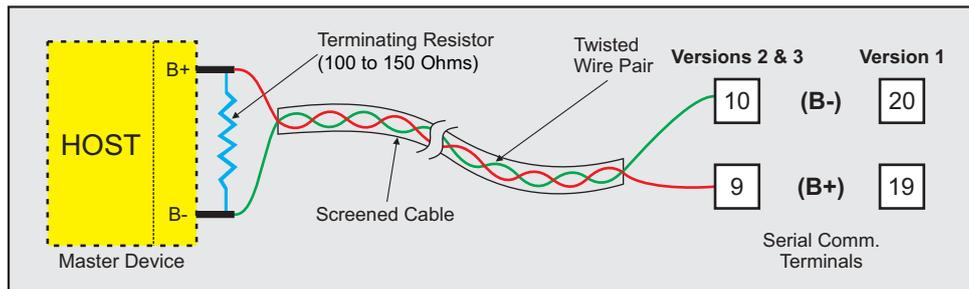
If the Optional plug-in communication board is fitted, connect terminals B+ and B- of the Indicator to the respective terminals of the Master device (PC/HMI). For reliable noise free communication, use a pair of twisted wires inside screened cable as shown in Figure 10.4. The wire should have less than 100 ohms/km nominal DC resistance (Typically 24 AWG or thicker). Connect the terminating resistor (Typically 100 to 150 ohm) at one end to improve noise immunity.
