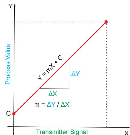
As is evident from the aforementioned transmitter examples, different transmitters produce signals varying both in *Type* (mV/V/mA) and *Range*. Most PPI instruments, thus, provide programmable Signal Type and Range to facilitate interface with a variety of transmitters. A few industry standard signal types and ranges offered by the PPI instruments are: 0-80mV, 0-5 V, 1-5 V, 0-10V, 0-20 mA, 4-20 mA, etc.
