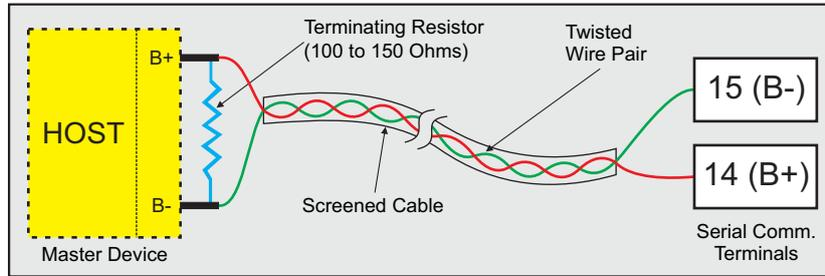
If the Optional plug-in communication board is fitted, connect terminal 15 and 14 of the indicator to (+) and (-) terminals of the Master device. For reliable noise free communication, use a pair of twisted wires inside screened cable as shown in Figure 3.6. The wire should have less than 100 ohms/km nominal DC resistance (Typically 24 AWG or thicker). Connect the terminating resistor (Typically 100 to 150 ohm) at one end to improve noise immunity.
