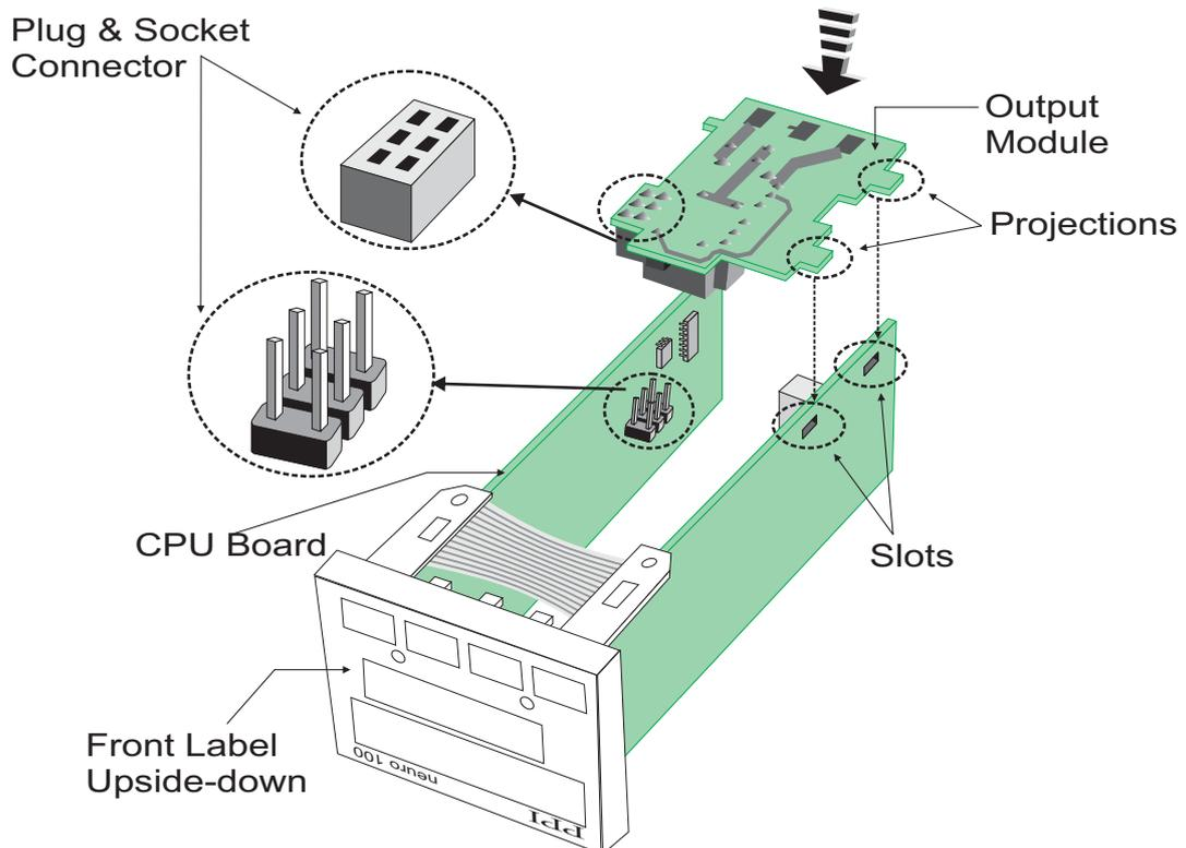
The plug for the Serial Communication or Remote Alarm Acknowledgment module is located on the Power-supply PCB. The Figure 9.7 below illustrates how to plug-in the Serial Communication/Remote Alarm Acknowledgment module. To plug (or unplug) the module simply insert (or remove) the socket into (or from) the plug.
