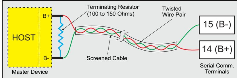
If the Optional plug-in communication board is fitted, connect terminal 15 and 14 of the indicator to (+) and (-) terminals of the Master device. For reliable noise free communication, use a pair of twisted wires inside screened cable as shown in Figure 11.6. The wire should have less than 100 ohms/km nominal DC resistance (Typically 24 AWG or thicker). Connect the terminating resistor (Typically 100 to 150 ohm) at one end to improve noise immunity.
